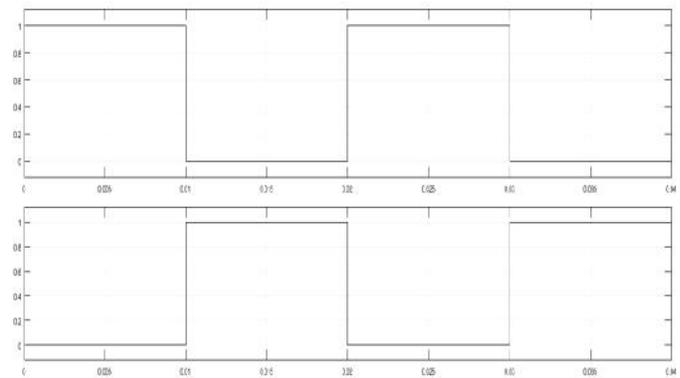
Figure 21. switching pulses for h-bridge
