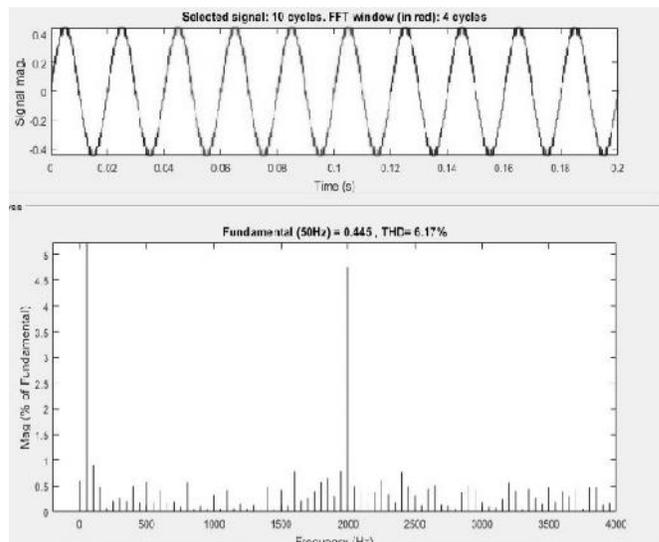
Figure 27. current thd for RL load (470 ohms, 20mh)
