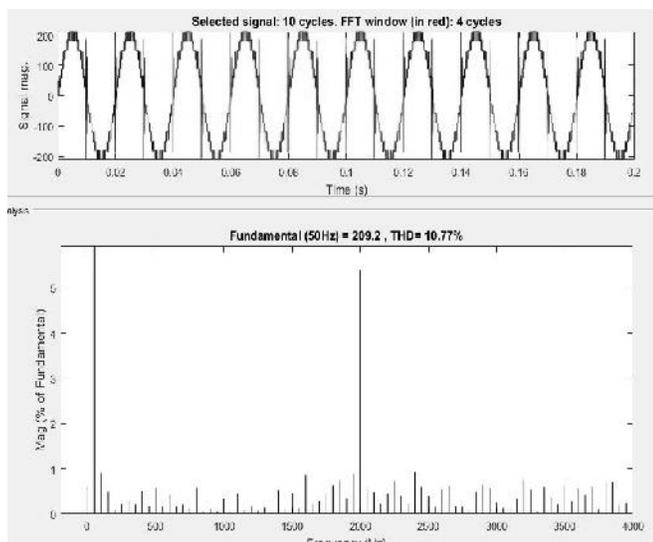
Figure 26. voltage thd for RL load (470 ohms, 20mh)
