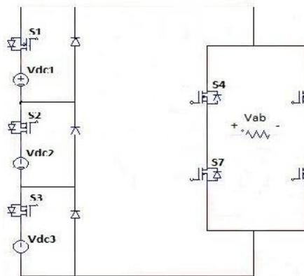
Figure 2. asymmetric h-bridge multilevel inverter
