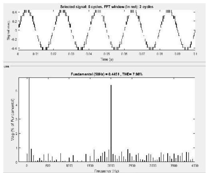
Figure 25. current thd for resistive load (470 ohms)
