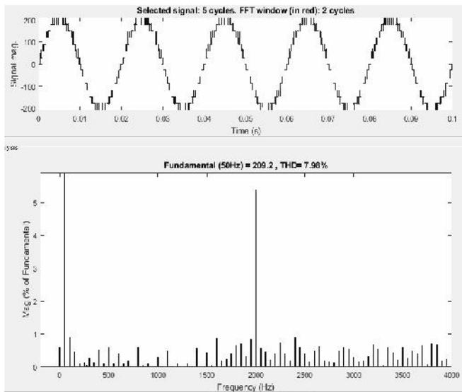
Figure 24. voltage thd for resistive load (470 ohms)
