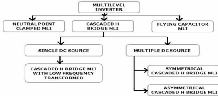
Figure 1. classification of multilevel inverters
