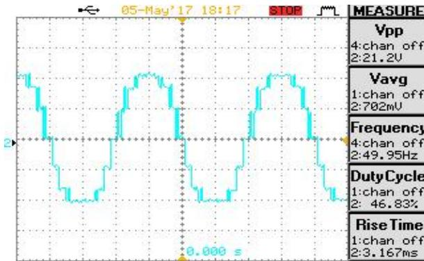
Figure 29. output voltage waveform of hardware circuit
