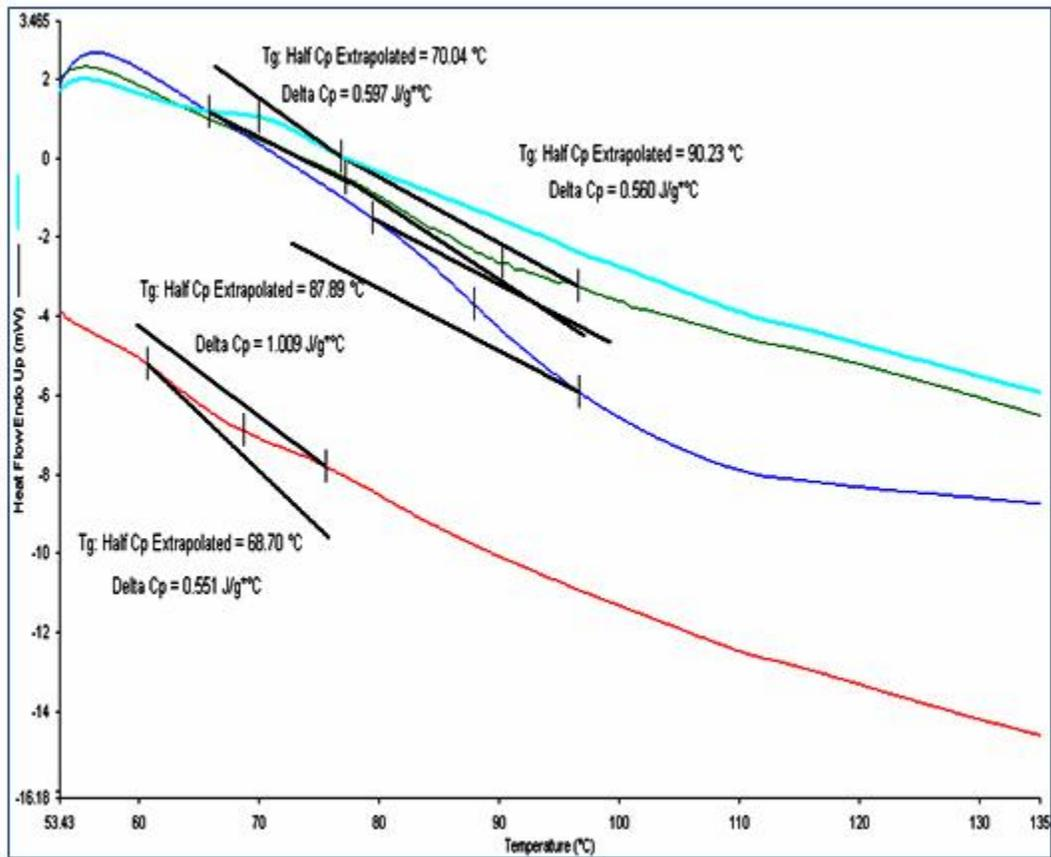
Figure 6. DSC Thermogram of CB-Epoxy composites for different weight % of CB
