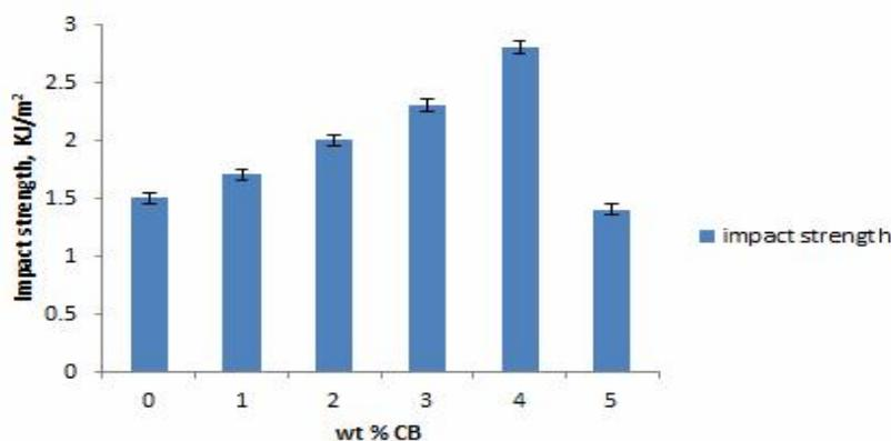
**Figure 5.** Impact strength of CB-Epoxy composites for different weight percentage of CB
