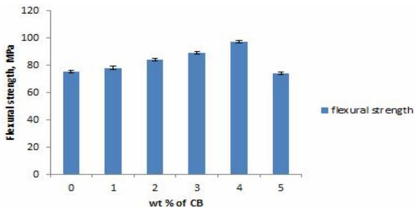
**Figure 3.** Flexural strength of CB-Epoxy composites for different weight percentage of CB
