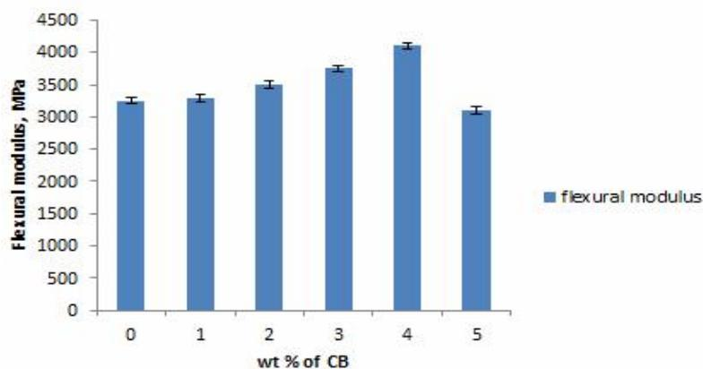
**Figure 4.** Flexural modulus of CB-Epoxy composites for different weight percentage of CB
