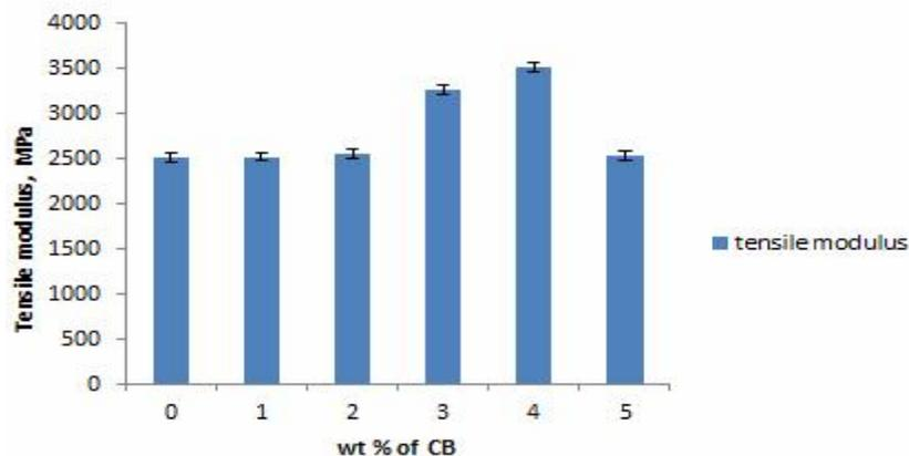
**Figure 2.** Tensile modulus of CB-Epoxy composites for different weight percentage of CB
