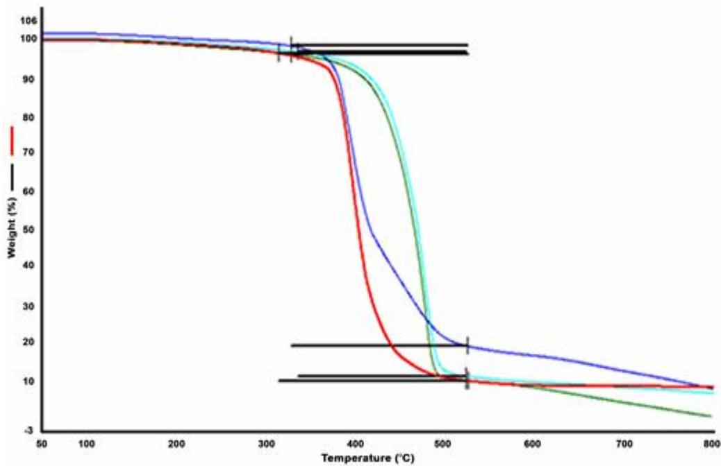
Figure 7. Percentage weight loss of the CB/epoxy composites due to heating in presence of N<sub>2</sub> atmosphere
