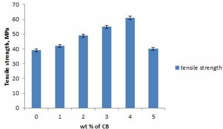
**Figure 1.** Tensile strength of CB-Epoxy composites for different weight percentage of CB
